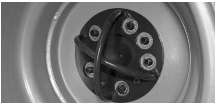
Tie down bracket on wheel hub A423091
